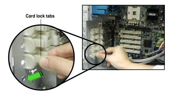
2. Firmly hold the expansion card and pull it out of the slot.
